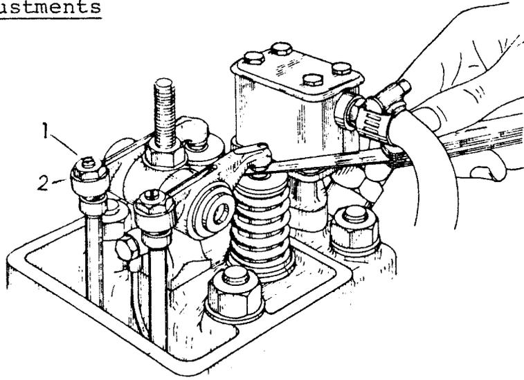
The valve clearance is to be adjusted when the engine is cold and should always be made after a re-tightening of the cylinder head. Further the valve clearance should be adjusted every 3 months.
