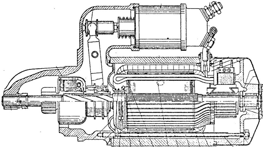
The starter motor is mounted on the left side of the engine seen from the flywheel end, and via a gear rim shrunk on the flywheel it starts the engine.
