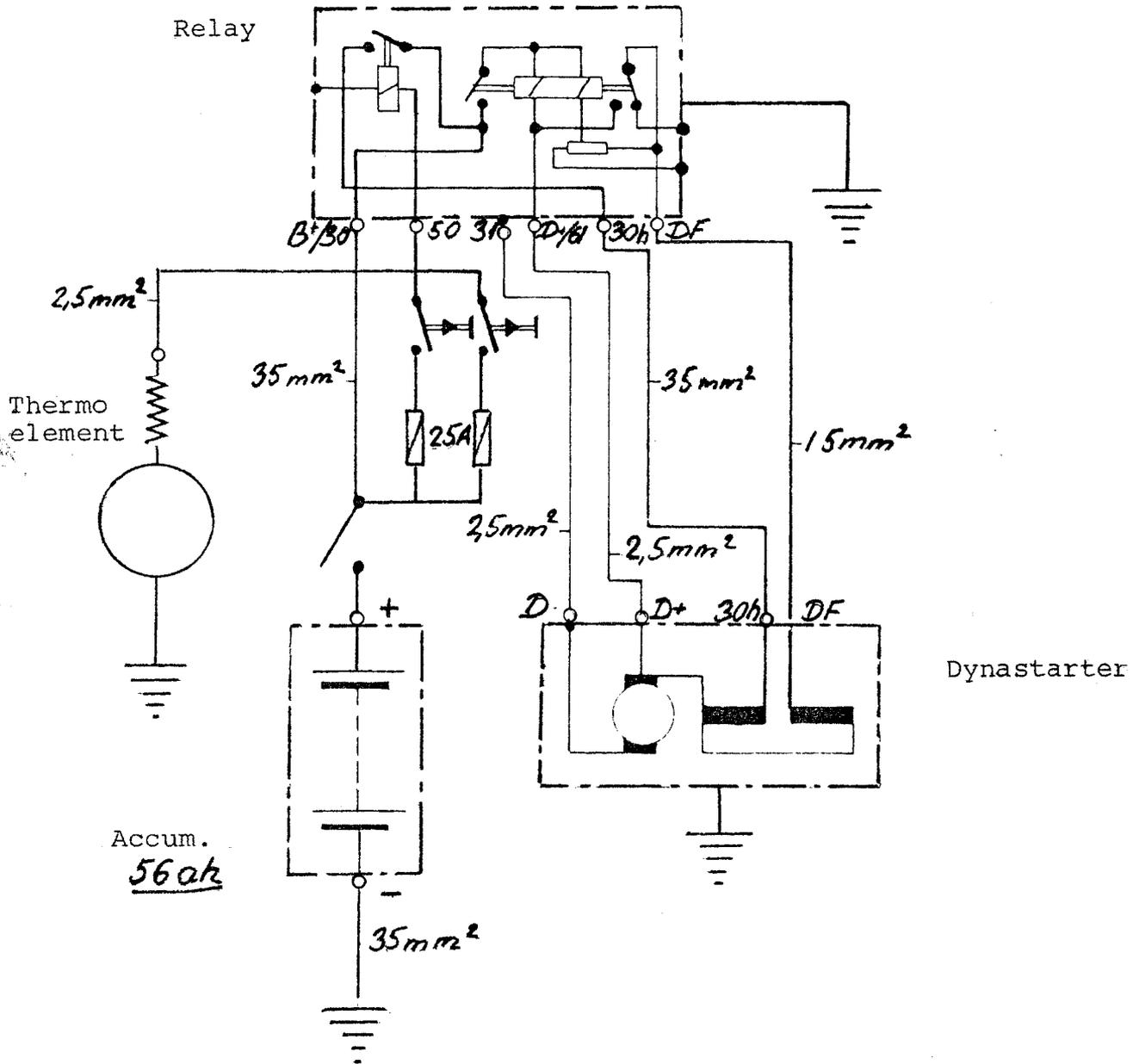
Wiring diagram for dynastarter with thermostart
