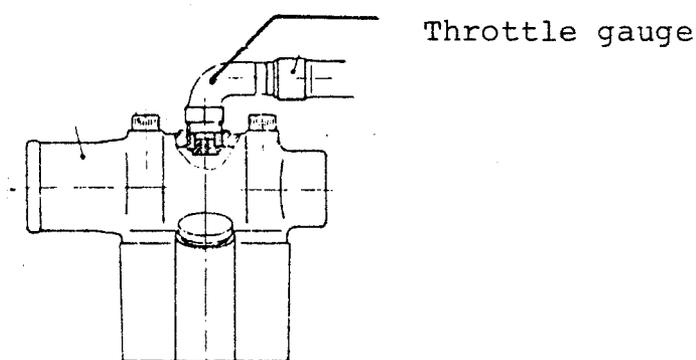
As shown on the above sketch a throttle gauge has been fitted in the cover in the venting connection. If this connection is choked the refrigerating capacity is considerably reduced owing to the increased quantity of air in the system.
