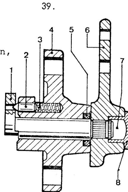
Press the shift control lever on to the shifter shaft so that shift control lever is placed in neutral position at  $90^{\circ} \pm 30'$  to the gear shaft length.
