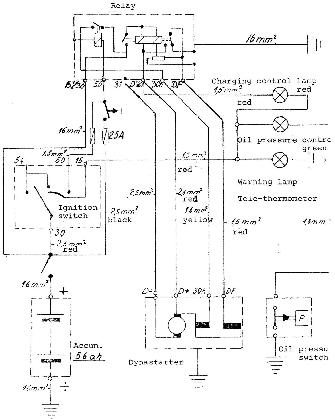
Wiring diagram for dynastarter with instrument panel.
