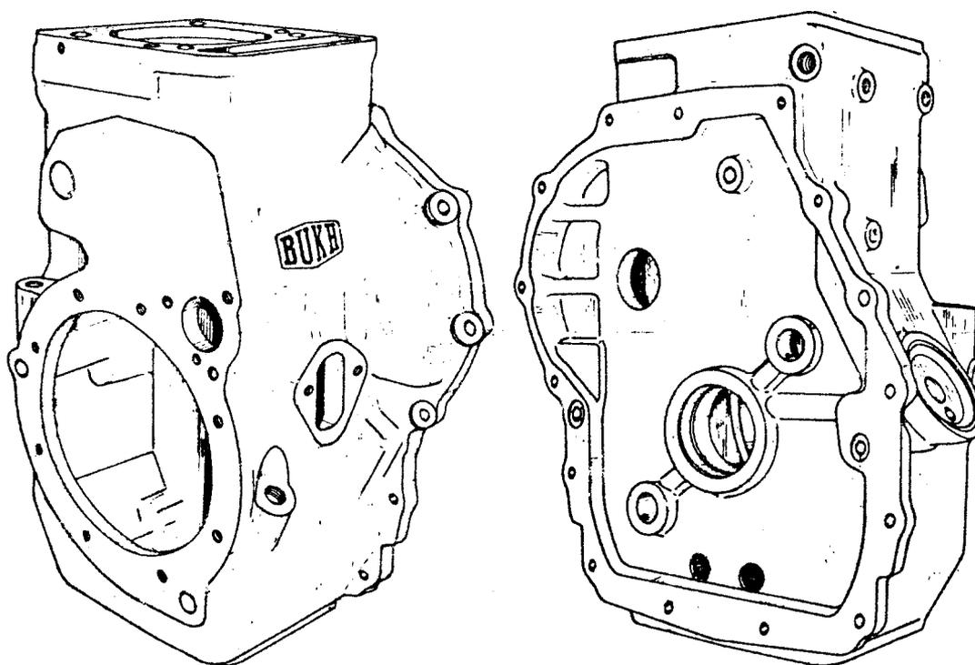
Placing of the bearing bush
