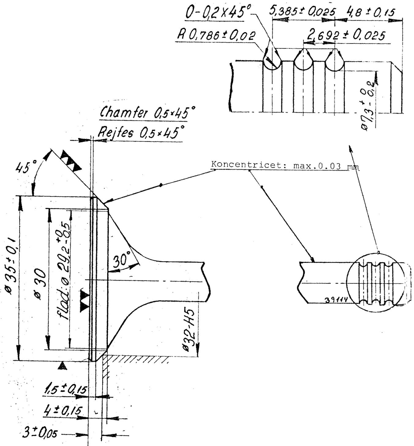
The seal face of the exhaust valve must max. have a breadth of 3.72 mm
