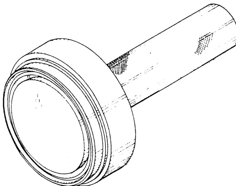
Mounting punch for oil seal ring.
