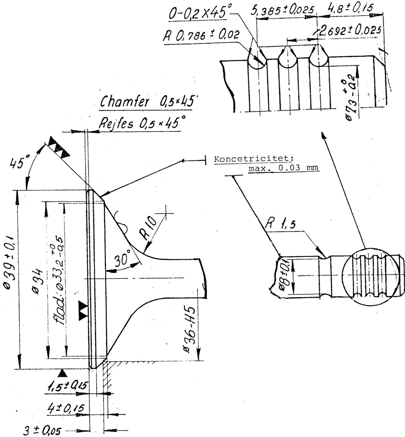
The seal face of the inlet valve must max. have a breadth of 3.72 mm.
