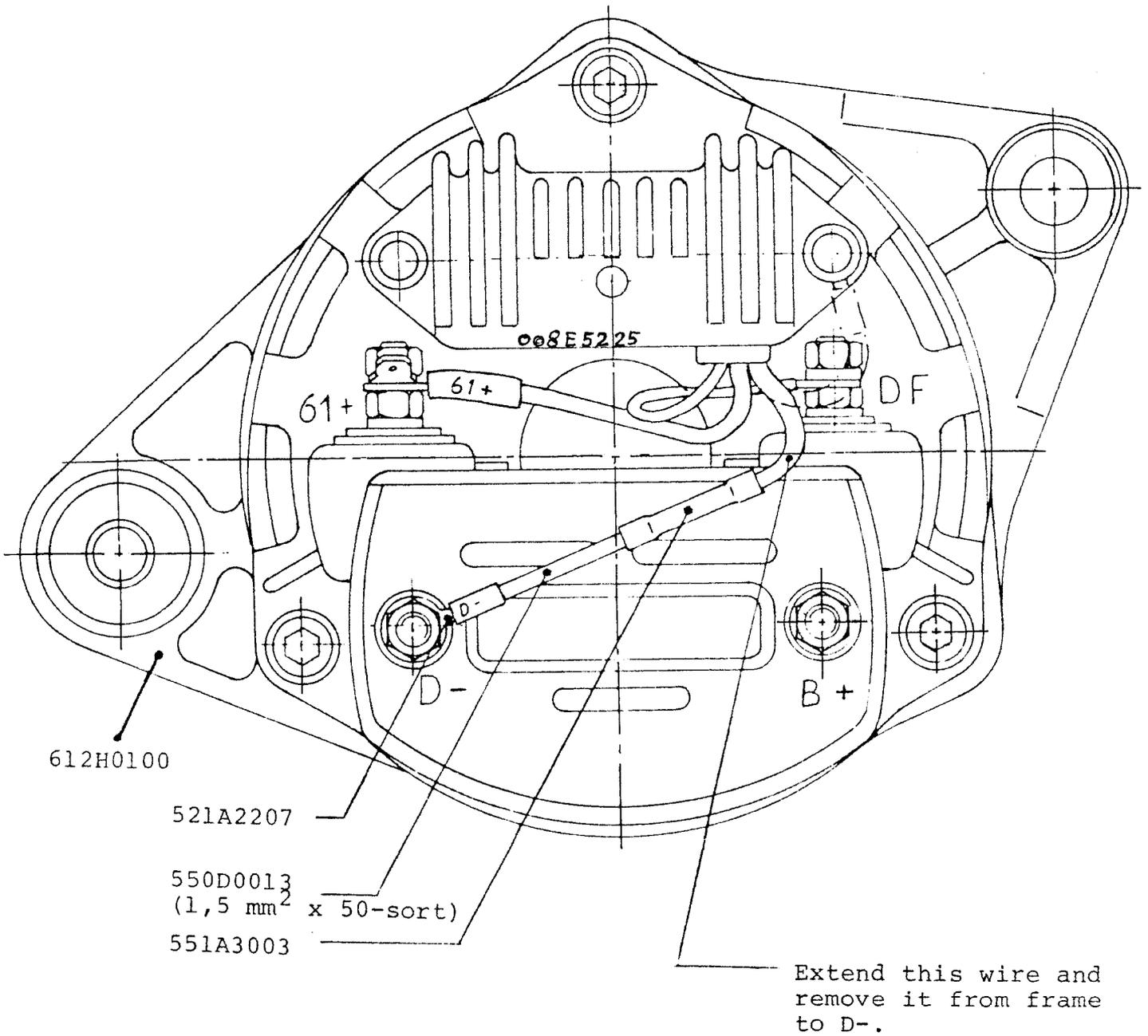
If the alternator is to be changed into 2-wire execution this should be carried out with the alternator dismantled from the engine.
