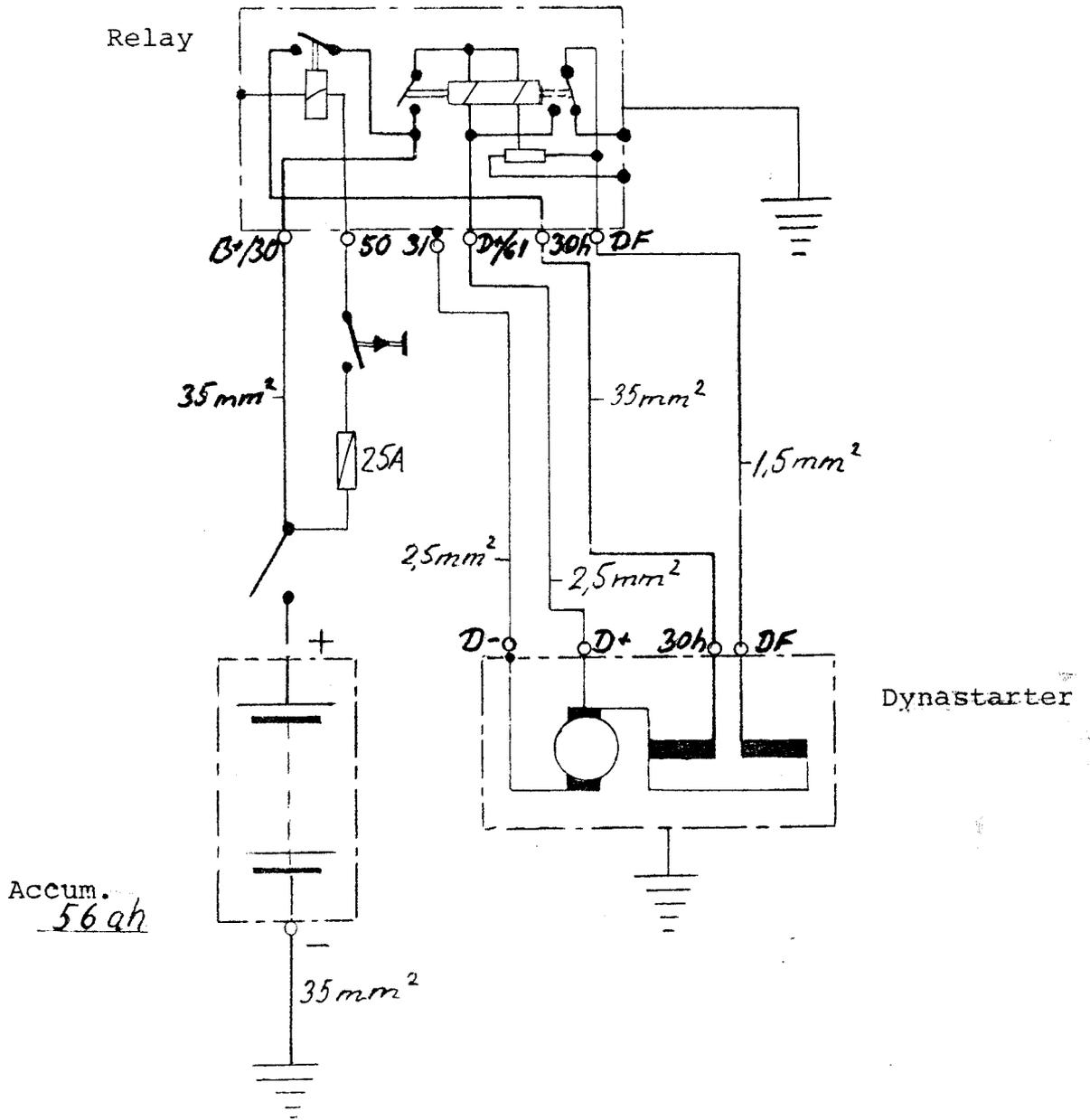
Wiring diagram for dynastarter
