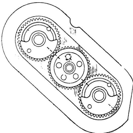
On new engine types mount the counterweight so that a tooth with one mark is facing a tooth space with one mark, and a tooth with two marks is facing a tooth space with one mark and a tooth space with two marks, respectively.
