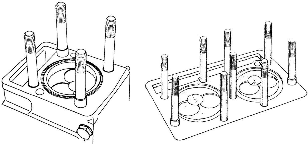
Tighten the cylinder head gasket to correct torque after about 25 operating hours. At the same time it is recommended to tighten the other gaskets of the engine.
