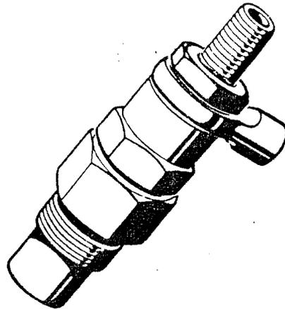
The fuel valve consists of injection nozzle and nozzle holder.
