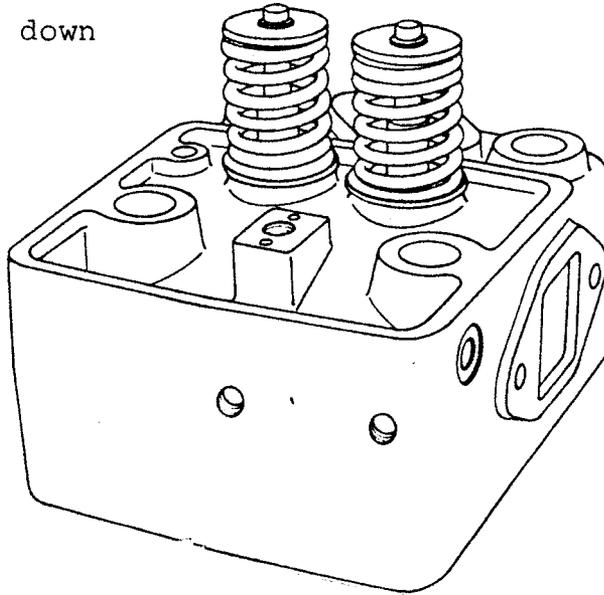
When mounting the valve springs you must take care that they are placed correctly - which can be seen from the above drawing.
