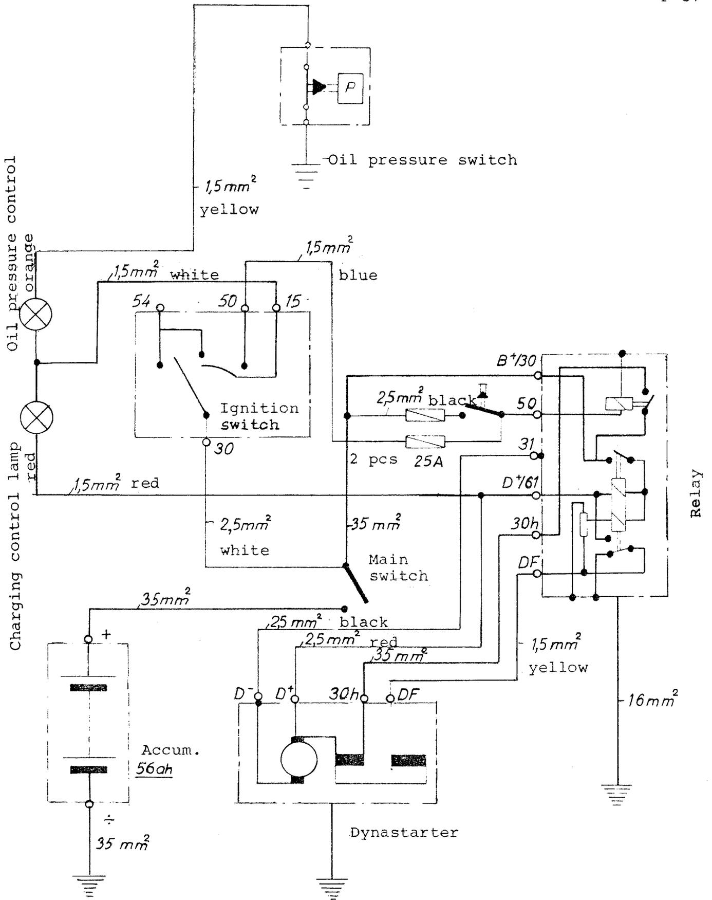
Wiring diagram for dynastarter with operating panel
