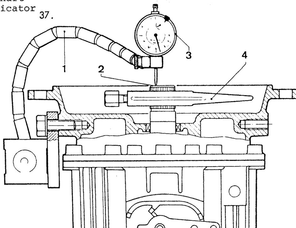
It would be an advantage, if the input shaft and the output shaft are measured individually for the adjusting of the tapered roller bearing tightening. The measuring procedure is the same both for input as well as for output. However, only the procedure for the input shaft is described here. When measuring the output shaft it should be as described at picture No. 31.
