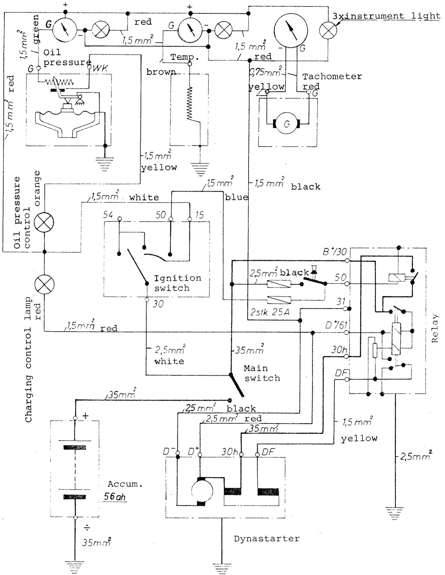
Wiring diagram for dynastarter with operating and instrument panel.
