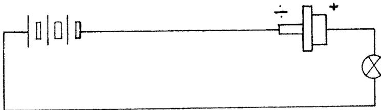
The measuring is carried out between the common base point (+) and the threaded rod (-) of the diode.
