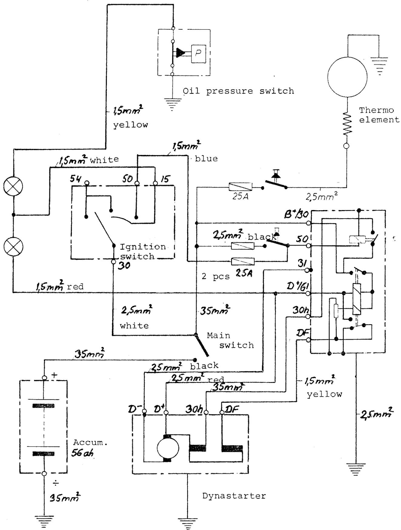
Wiring diagram for dynastarter with thermostart and operating panel
