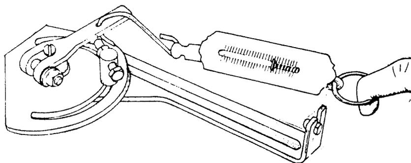
1. Adjust the tightness of the governor arm by altering the number of disk springs below the regulating quadrant.
