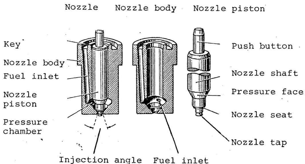
When working with fuel valves and their nozzles observe the greatest cleanliness, and all parts must be washed and cleaned carefully with pure petrol at the dismantling.
