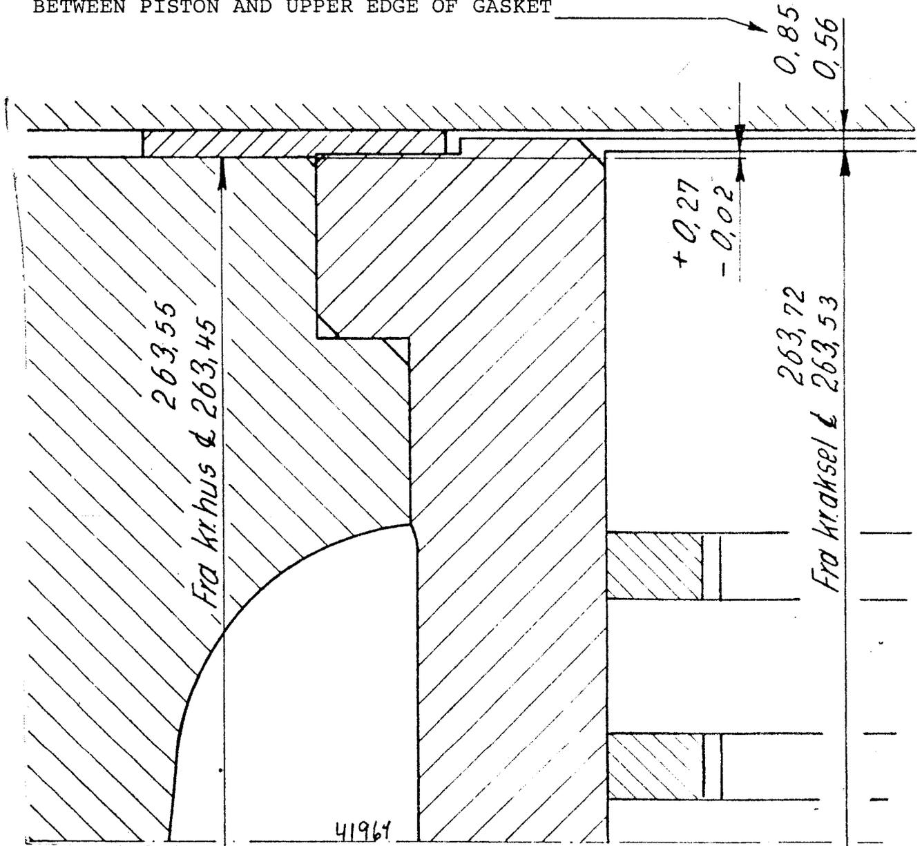
TEST MEASUREMENT OF CYLINDER LINER
