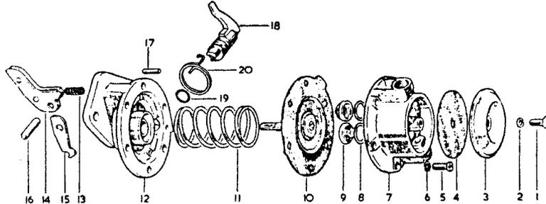
The fuel pump can be dismantled as shown on the drawing, but in cases where more parts than for instance the valves or the diaphragm must be replaced it will often pay to mount a new pump as these are very cheap to purchase.
