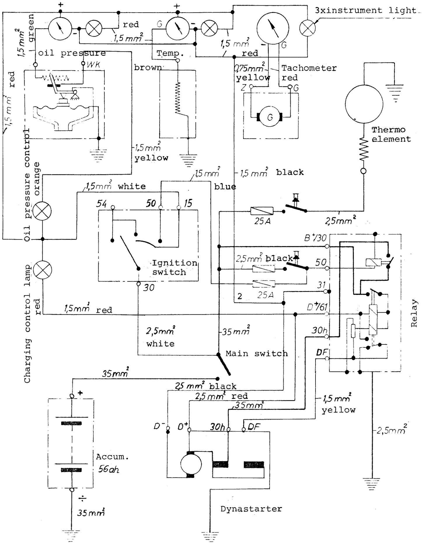
Wiring diagram for dynastarter with thermostart plus operating and instrument panel,
