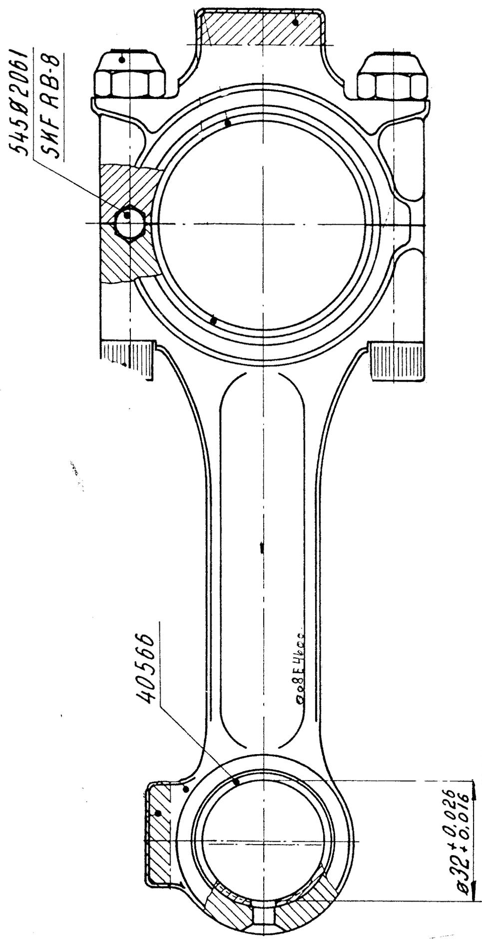
CALIBRATE WITH BALL AFTER PRESSING-IN OF LINING
