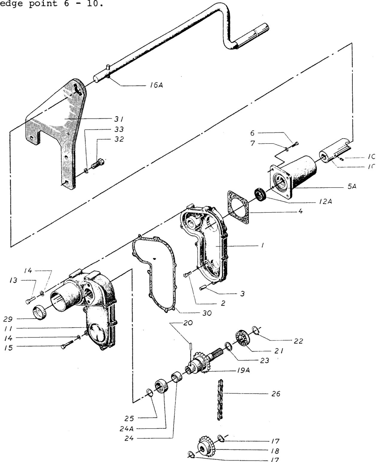
Arrangement of raised hand start on rear edge
