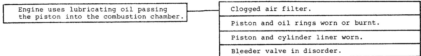
9. EXCESSIVE LUBRICATING OIL CONSUMPTION
