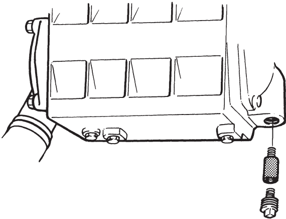
TAMD63: Zinc anode in heat exchanger's front end cover
