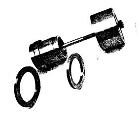
Lining-up tool for intermediate guard (dial micrometer not included).
