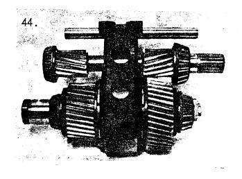
Fit intermediate wheel and needle bearing.
