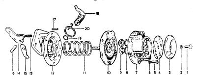
The fuel pump can be dismantled as shown on the drawing, but in cases where more parts than for instance the valves or the diaphragm must be replaced it will often pay to mount a new pump as these are very cheap to purchase.
