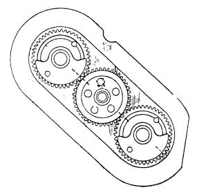
On new engine types mount the counterweight so that a tooth with one mark is facing a tooth space with one mark, and a tooth with two marks is facing a tooth space with one mark and a tooth space with two marks, respectively.
