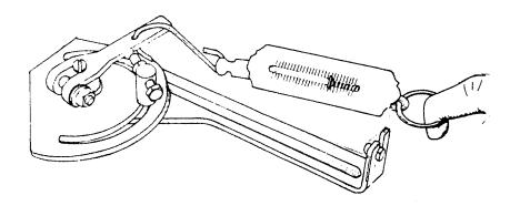
Adjust the tightness of the governor arm by altering the number of disk springs below the regulating quadrant.
