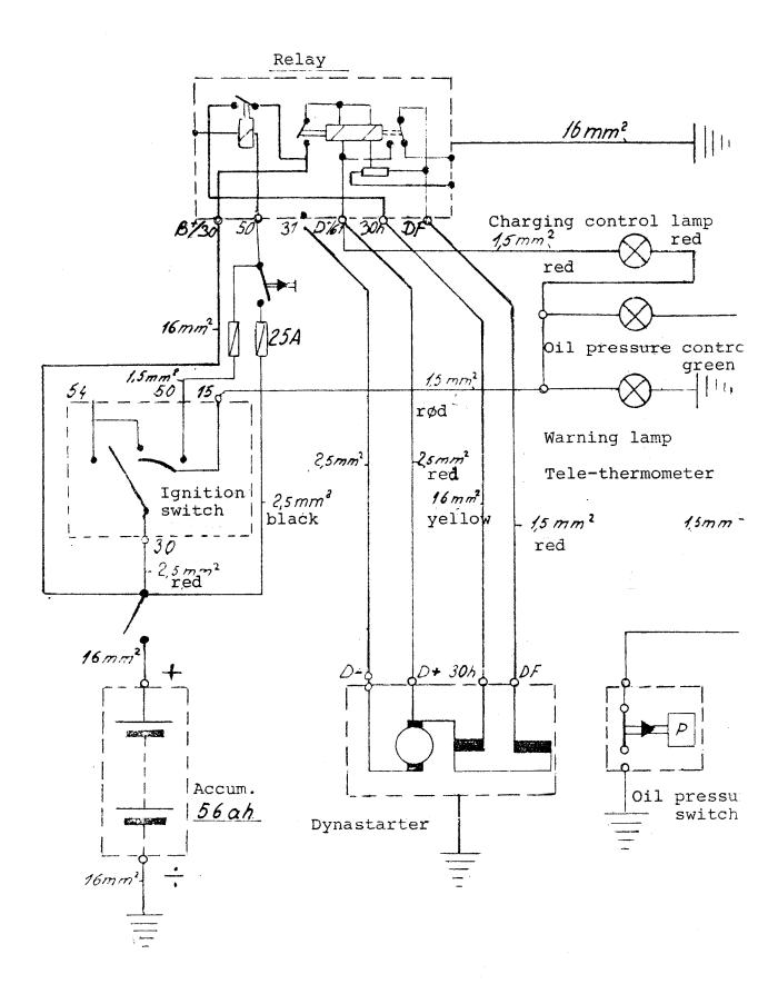
Wiring diagram for dynastarter with instrument panel
