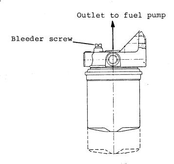
From the above engine Nos. the fuel filter has been altered to a throw-away filter.
