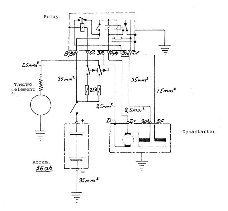
Wiring diagram for dynastarter with thermostart
