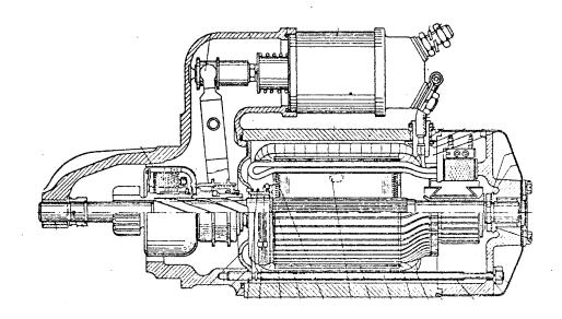
The starter motor is mounted on the left side of the engine seen from the flywheel end, and via a gear rim shrinked on the flywheel it starts the engine.
