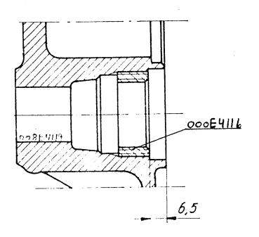
2. Smear READIT 5850 on the threaded piece No. 000E4116 on the external thread and fit it by means of the tool No. 008E4224. The threaded piece must be tightened the whole way down.
