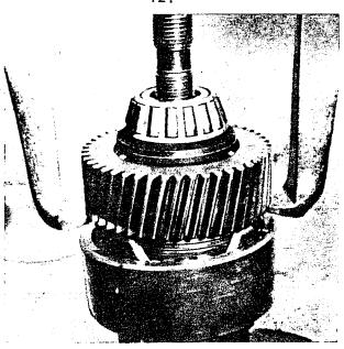
Remove thrust collar with bolts and washers together with needle bearing bushing, sliding sleeve and pressure spring.
