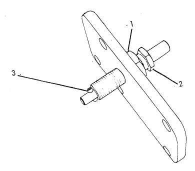
The stop button is correctly adjusted from the factory. At possible repairs it will not be necessary to readjust. In case of dismantling of stop button this is carried out as follows:
