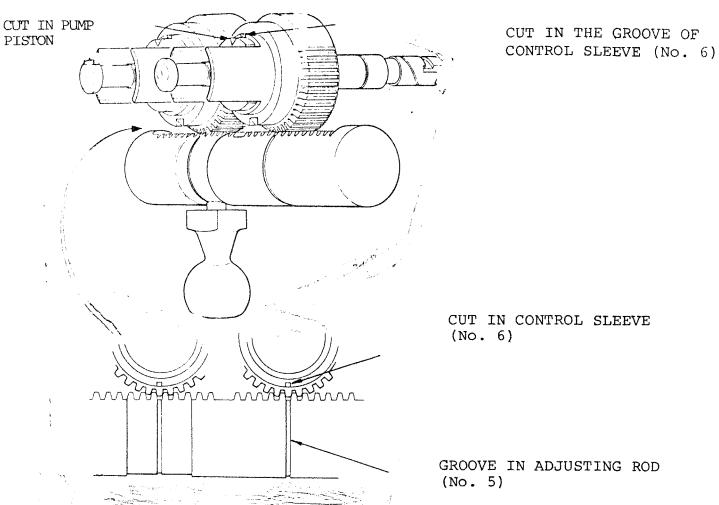
MESH FOR CONTROL SLEEVE AND ADJUSTING ROD
