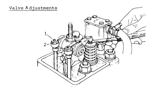
The valve clearance is to be adjusted when the engine is cold and should always be made after a re-tightening of the cylinder head. Further the valve clearance should be adjusted every 3 months.
