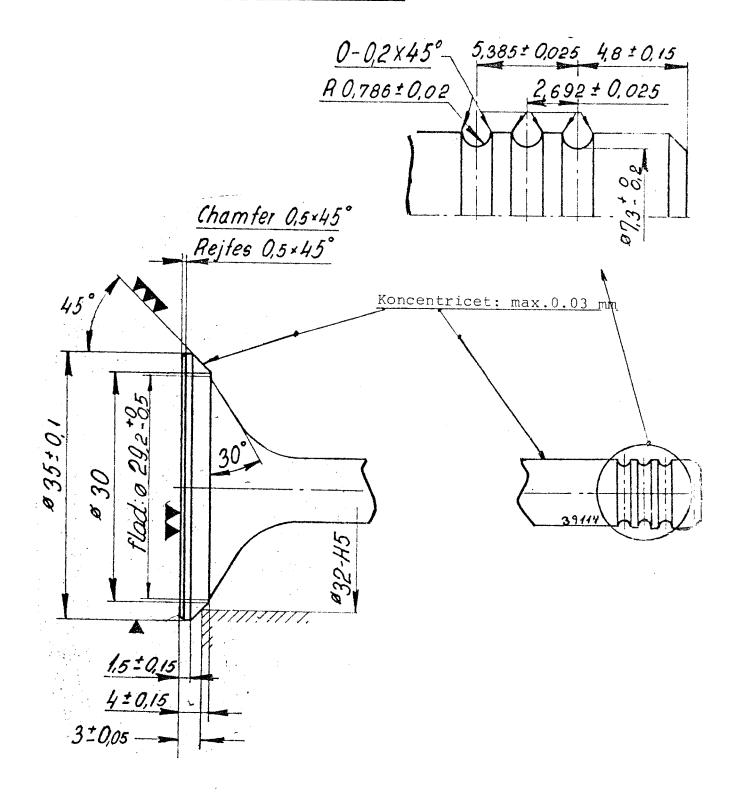
The seal face of the exhaust valve must max. have a breadth of 3.72 mm
