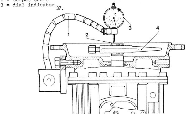
It would be an advantage, if the input shaft and the output shaft are measured individually for the adjusting of the tapered roller bearing tightening. The measuring procedure is the same both for input as well as for output However, only the procedure for the input shaft is described here. When measuring the output shaft input as well as for output it should be as described at picture No. 31.
