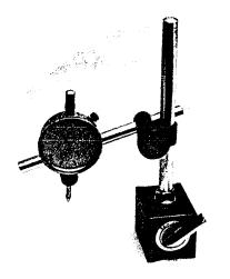
Dial micrometer with magnetic holder. For use in adjusting spill point and lining-up of intermediate guard.
