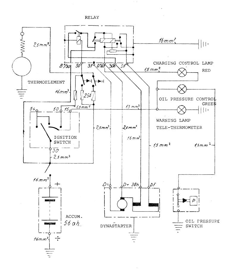
Wiring diagram for dynastarter with thermostart and instrument panel.
