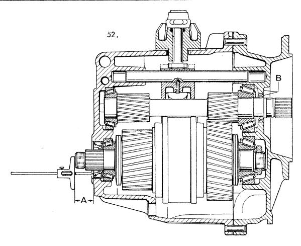
A = distance to shaft seal ring 22.5 +/- 0.5 mm.
