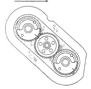
On old engine types mount the counterweight so that the marked tooth on the crankshaft gear-wheel is facing the mark on the counterweight.
