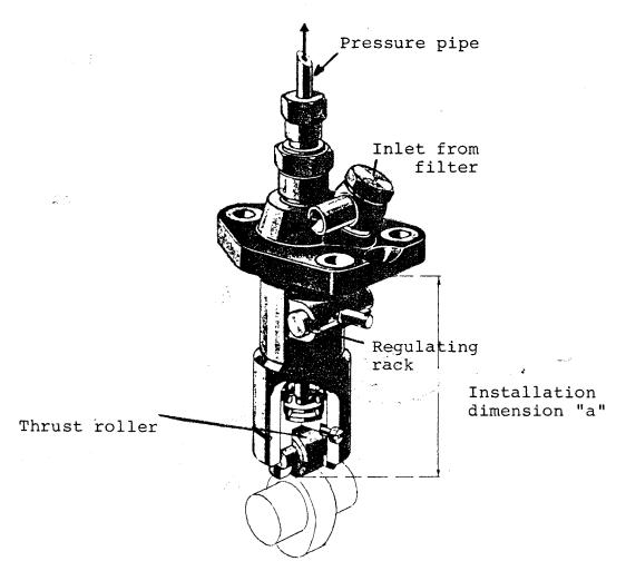
The fuel pump is a single-acting piston pump activated by the fuel cam of the camshaft through a roller guide. A spring built into the pump housing secures that the pump piston and the spring are constantly pressed against the fuel cam.
