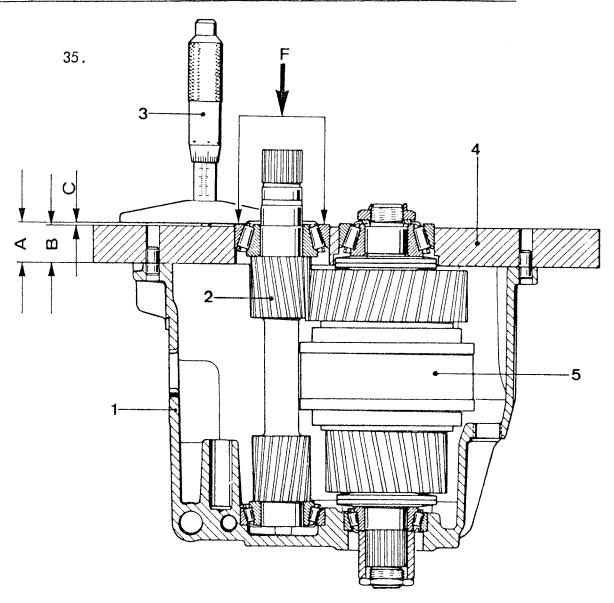
1 = house 3 = depth micrometer 5 = output shaft 2 = input shaft  $4 = \text{measuring gauge } 1 \times 56 \times 136 \times 978$   $6 = 30 \times (3.0 \text{ kp})$
