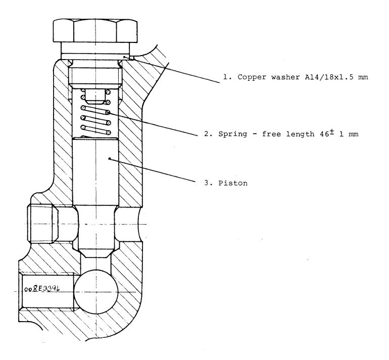
The above fig. Nos. show the lubricating oil reduction valve in the new execution. The improvement is that the designing of the valve has been changed. The function is still the same.
