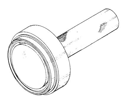
Mounting punch for oil seal ring.
