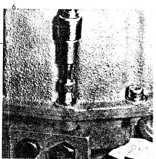
Drive back the fitting pins 2 -3 mm in the gearbox and lift one gearbox half with reversing shaft, input and output shafts free of the other gearbox half.
