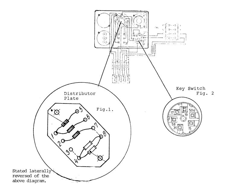
Three diodes (type IN4002 - BUKH No. 552A2102) are fitted on the distributor plate. Of these three diodes the two upper ones see to it that the lamp with alarm is alight and that the connection for this lamp is connected with the acoustic alarm at the same time. The bottom diode is inserted so that it actuates the acoustic alarm, if the key is left in pos. 58 in the key switch, where the stop solenoid is actuated.
