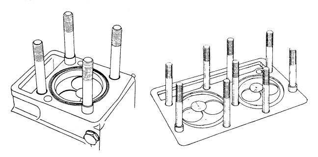
Tighten the cylinder head gasket to correct torque after about 25 operating hours. At the same time it is recommended to tighten the other gaskets of the engine.
