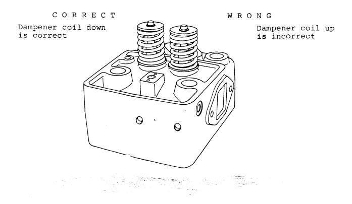
When mounting the valve springs you must take care that they are placed correctly - which can be seen from the above drawing.
