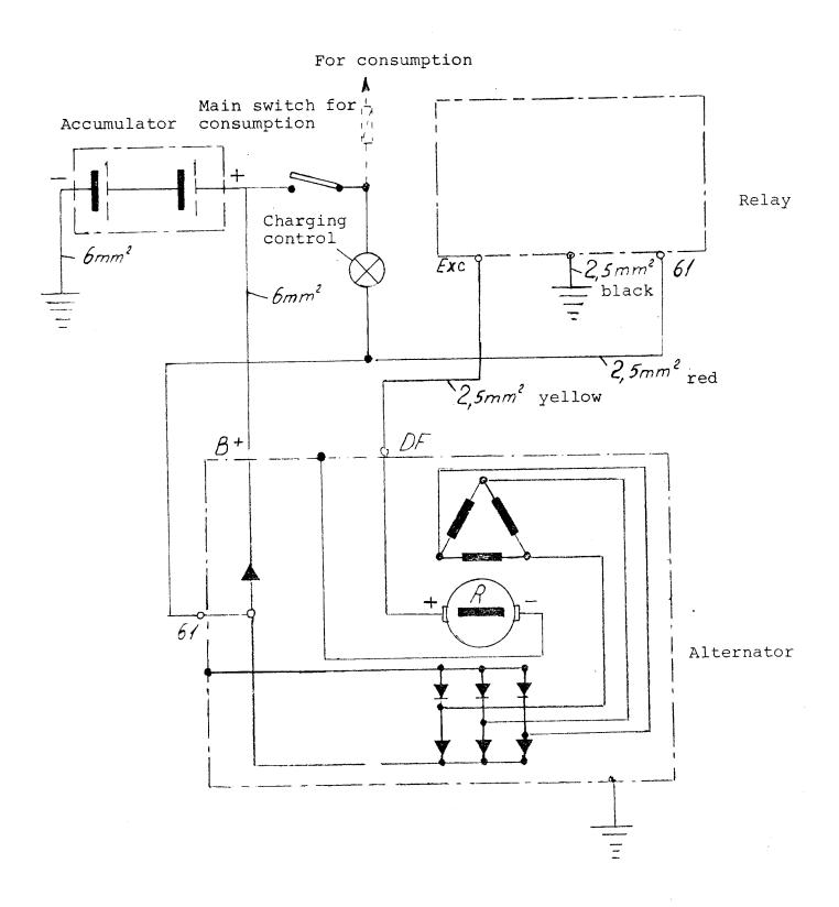
Wiring diagram for alternator
