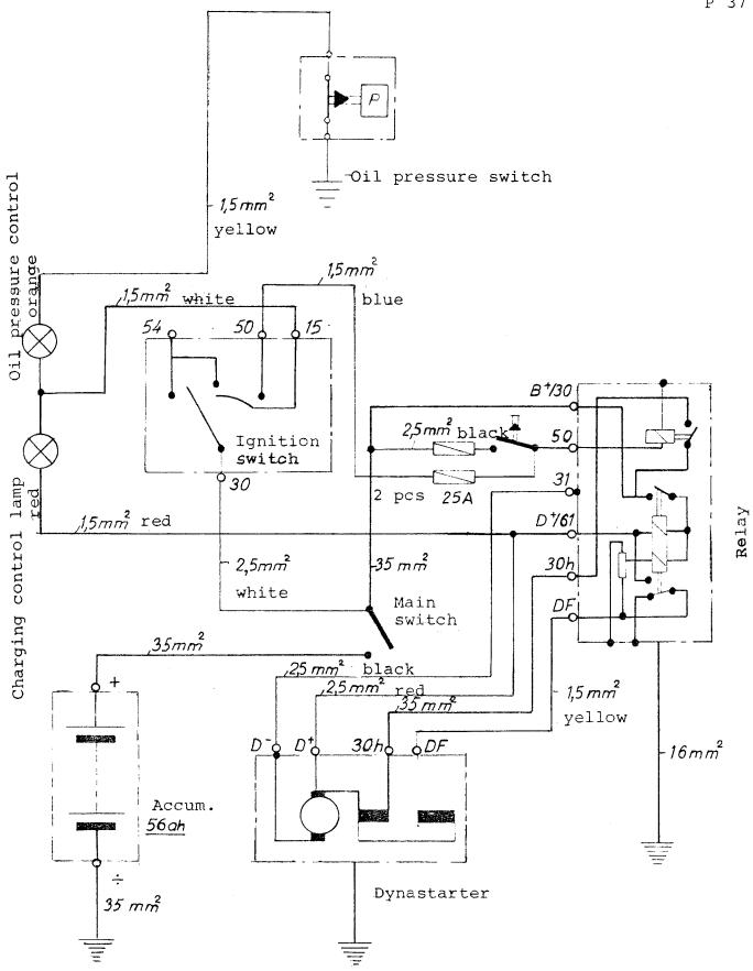
Wiring diagram for dynastarter with operating panel
