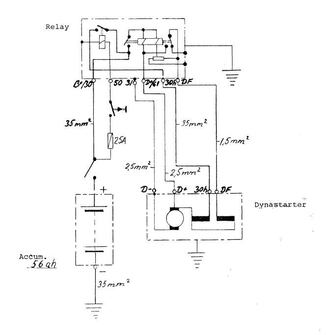
Wiring diagram for dynastarter
