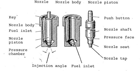
When working with fuel valves and their nozzles observe the greatest cleanliness, and all parts must be washed and cleaned carefully with pure petrol at the dismantling.
