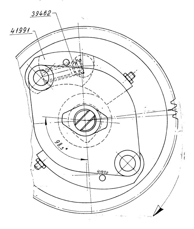
Please Note: Fitting of the injection timer in proportion to the gear-wheel mark.
