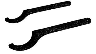
Tools for removing and fitting main bearings
