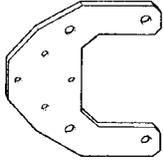
885224-6 Engine fixture. The tool should be supplemented with 4 pcs pin screws 479971-4, 4 pcs nuts 971095-5, 4 pcs screws 970964-3 (M10x140), 4 pcs screws 955311-6 (M8x140), 4 pcs washers 960148-5 (M10), 4 pcs washers 960141-0 (M8) and the arms from engine fixture 885050-5.
