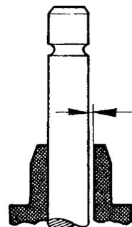
Fig. 22. Clearance, valve - valve guide (cylinder head)
