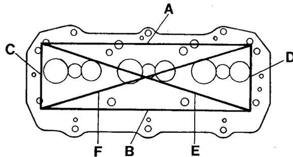
Fig. 16. Checking of cylinder head flatness
