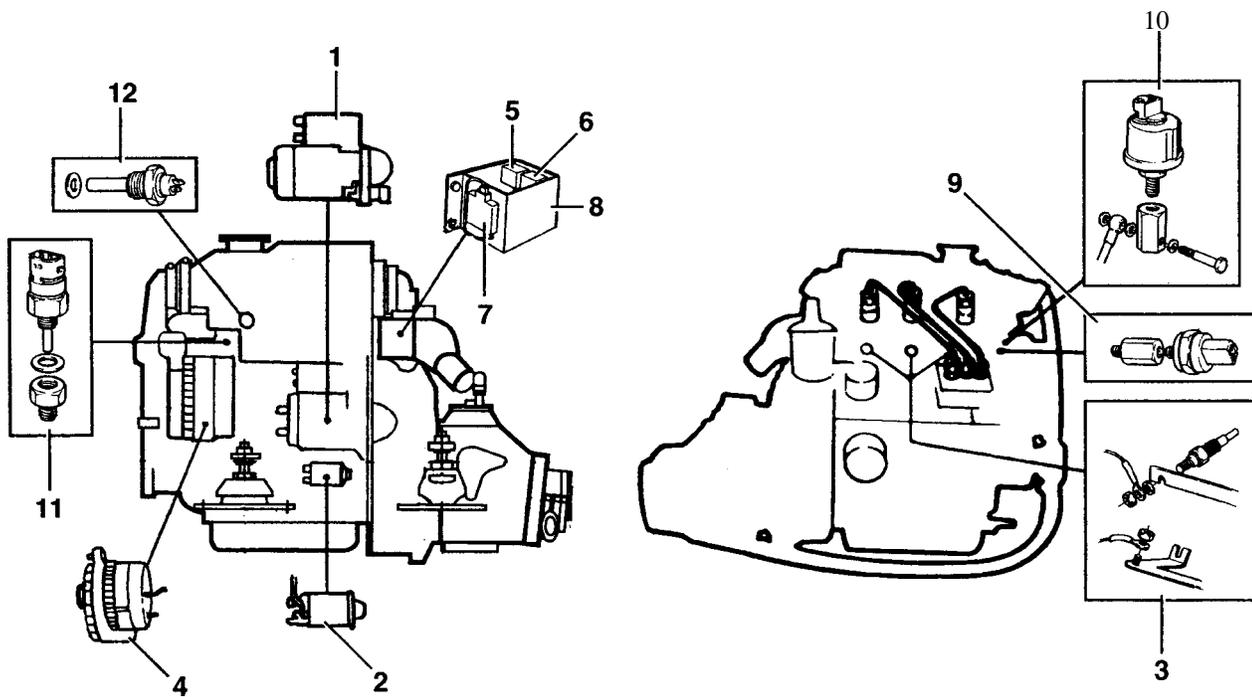
Fig. 111. Positioning of electrical components on the engine
