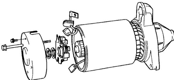
Fig. 116. Dismantling of the bearing shield
