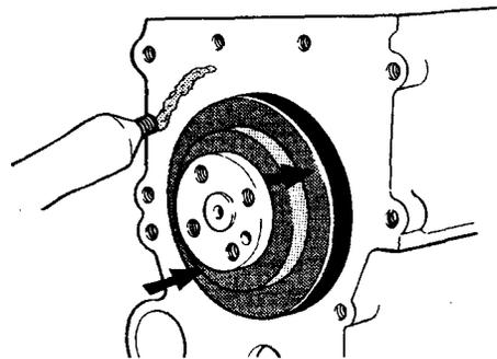
Fig. 81. Fitting of crankshaft seal
