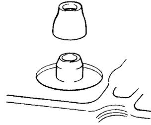
Fig. 28. Fitting of valve stem seals
