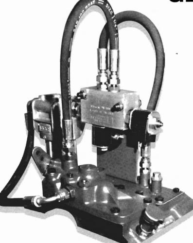
The Newage trolling valve enables low propeller speeds to be obtained by the use of an electrically controlled pressure reducing valve in the clutch pressure operating circuit.
