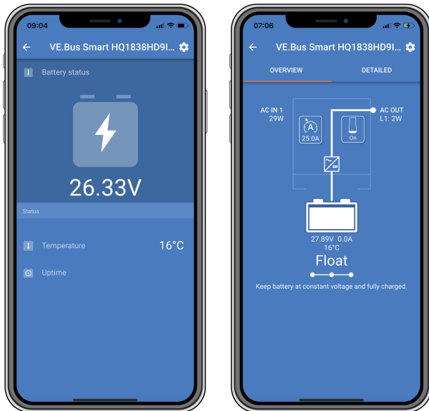
VictronConnect screens without and with inverter/charger connected.
