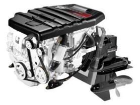
Fuel System: Bosch Common Rail (CRS 2.0);
