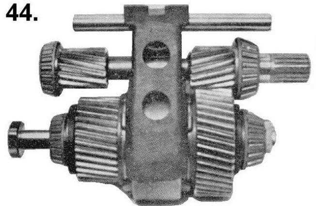
Fit the intermediate wheel and needle bearing.
