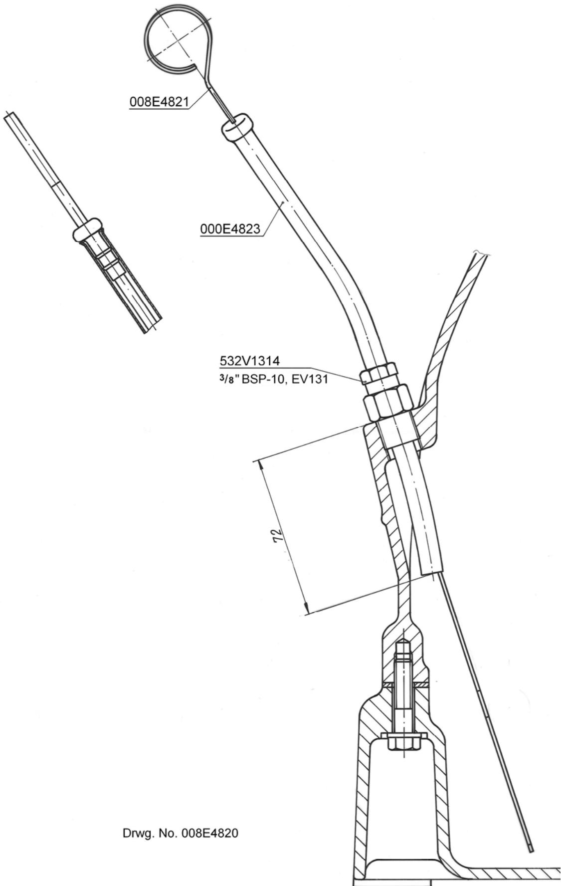
Pipe connections in oil sump
