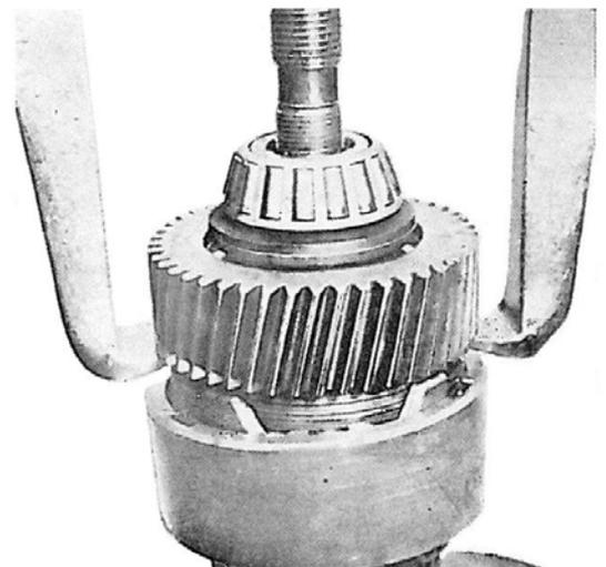
Remove the thrust collar with bolts and washers together with needle bearing bushing, sliding sleeve and pressure spring.
