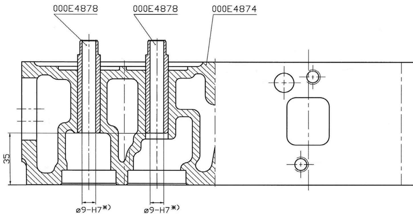
\* ) The valve guides tolerance after fitting
