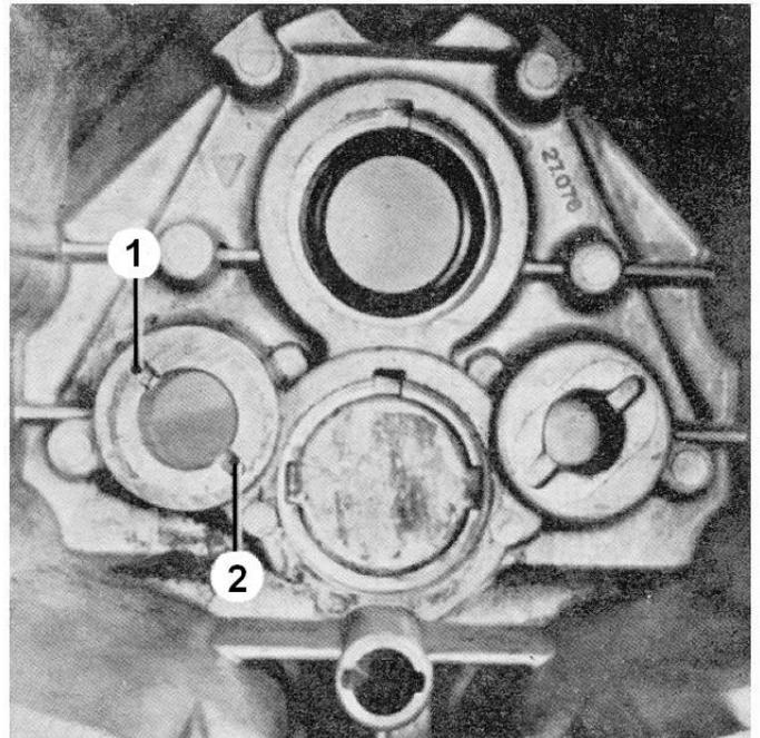
Heat the gearbox and fit the bolts with slotted pins in pos. 1 or 2 all depending on the transmission.
