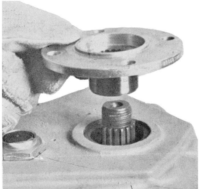
Smear the nut with permanently plastic liquid jointing and secure it with a torque of 100 Nm ( 10 Kpm).
