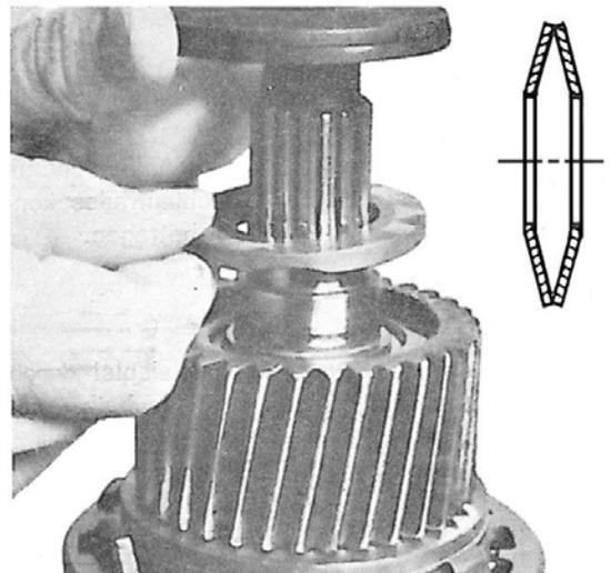
Check the tightening of the disc springs.
