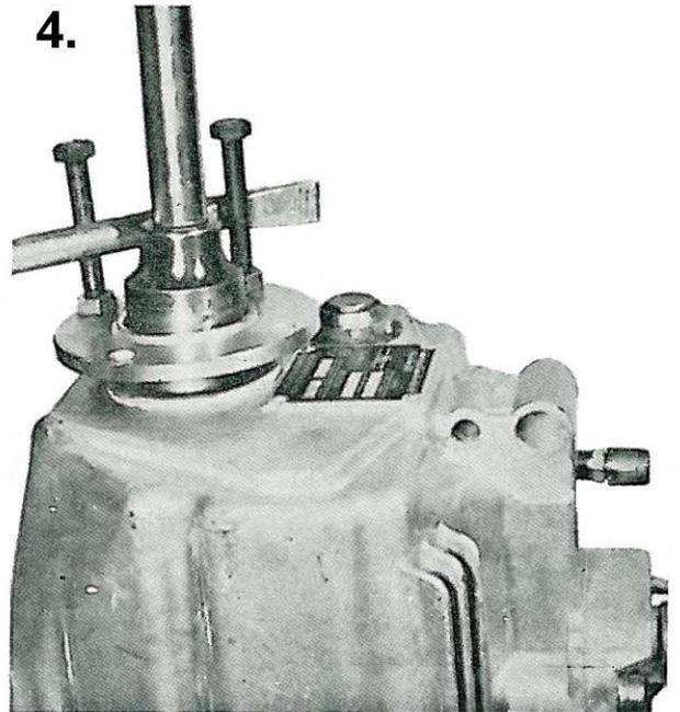
Pull off the output shaft flange.
