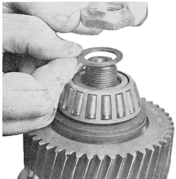
The picture shows the ready-mounted output shaft.
