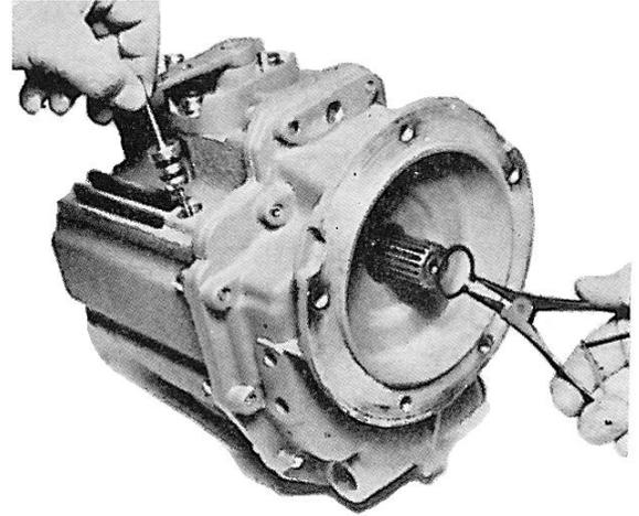
Remove the shifting arrangement with gasket.
