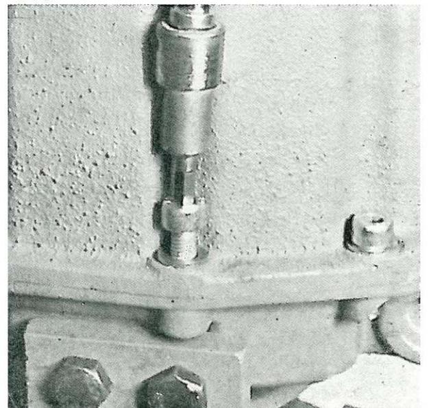
Drive back the fitting pins 2 – 3 mm in the gearbox and lift one gearbox half with reversing shaft, input and output shafts free of the other gearbox half.
