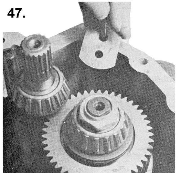
Smear the seal faces of the gearbox halves with permanently plastic liquid jointing.
