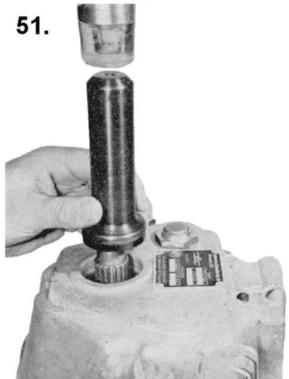
Supplement to Fitting of Shaft Seal Rings
