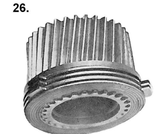
Fit wheel for "AHEAD" with clutch discs on the thrust collar.
