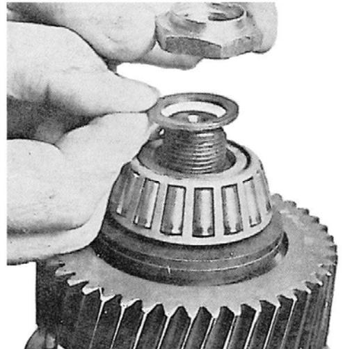
Pull off the wheel "ASTERN" with a special tool and take up washer, disc springs and tapered roller bearing inner collar.
