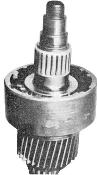
Remove the wheel "AHEAD" with a special tool and take off all parts "AHEAD".
