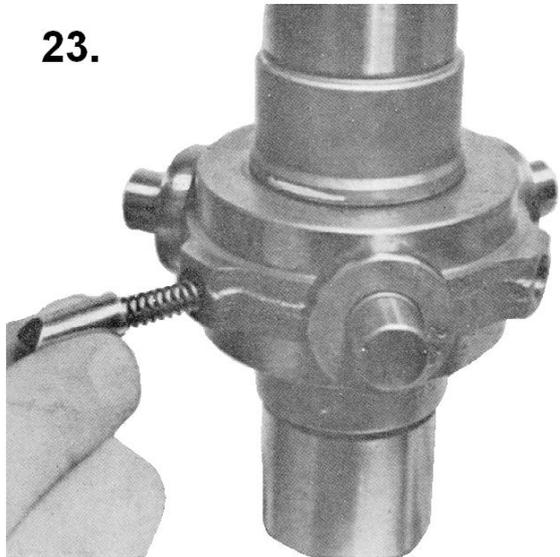
Press the sliding sleeve from the bottom against the check bolts.
