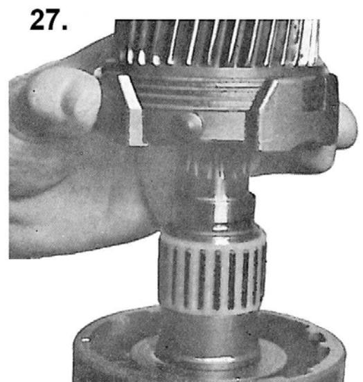
Fit thrust washer, the oil pockets of which should turn towards the wheel for "AHEAD".
