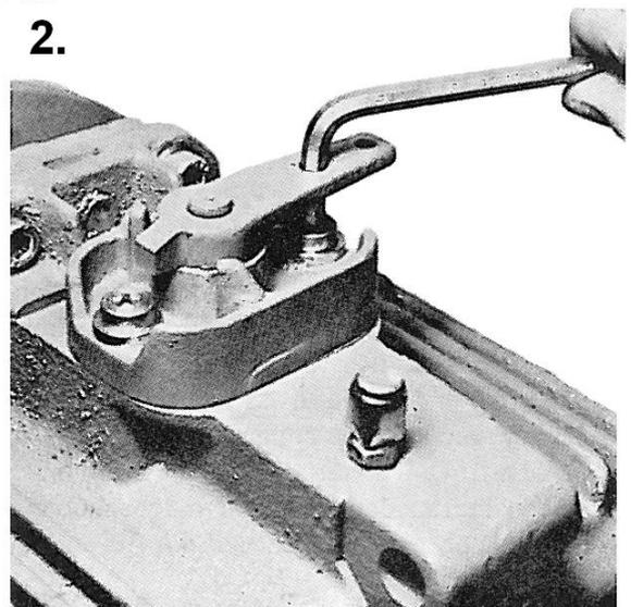
There are two different shifting levers which, however, can be built in without any problems in either cases.
