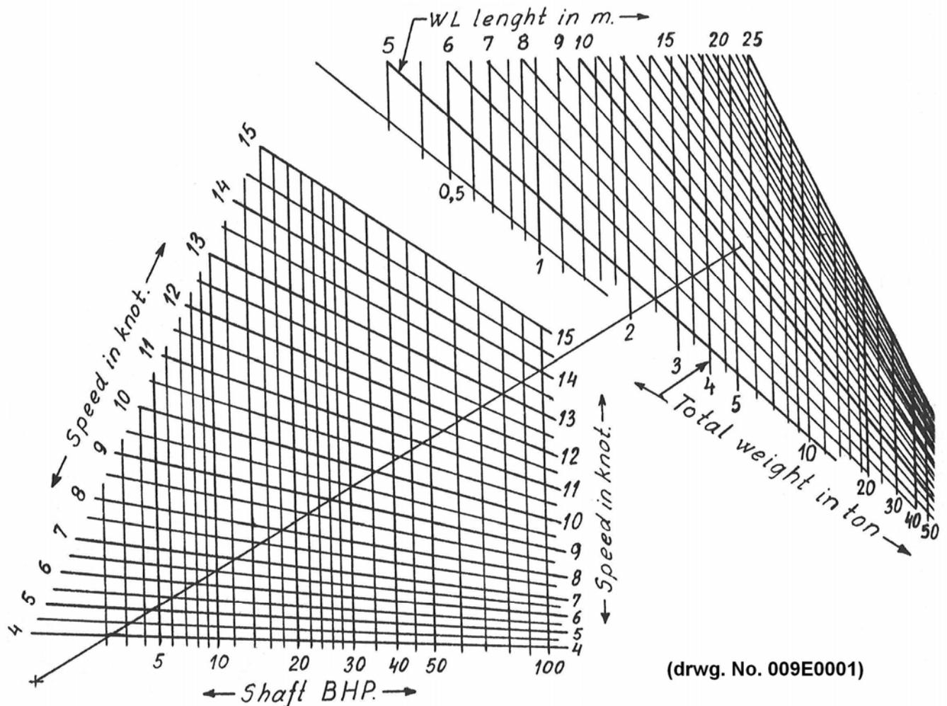
Seek the scheme to the right of the intersection between the actual length in the waterline of the ship and the total weight.
