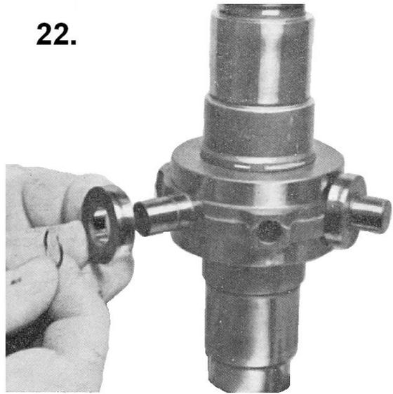
Fit the pressure springs in the check bolts. Fit the check bolts in the corresponding bores.
