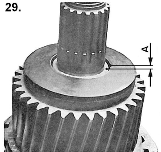
Tighten the disc springs with bush 1 x 56 136 994. Measure disc clearance between inner disc and washer with a feeler gauge in two places which are opposite one another.
