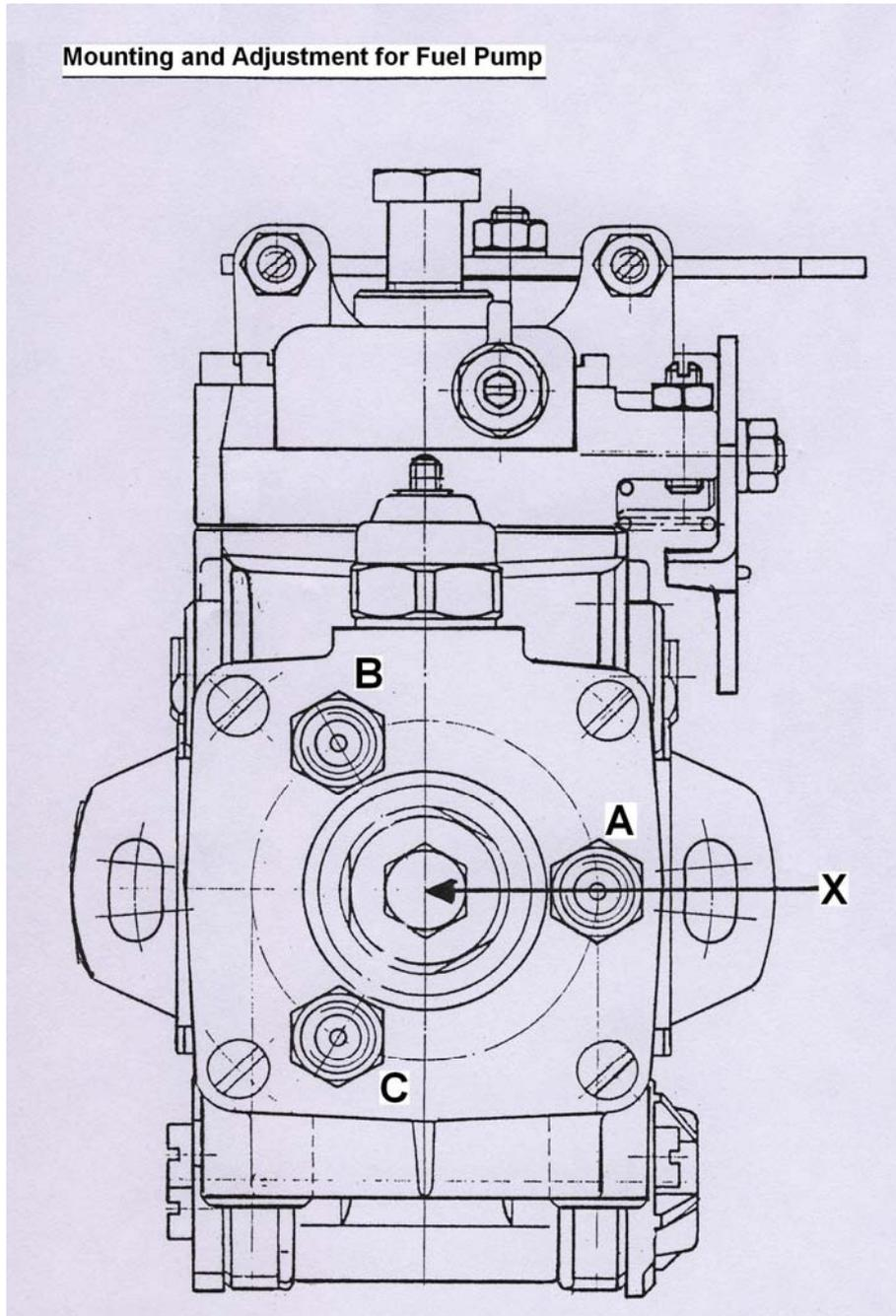
1. Turn piston No. 3 (rear) to TOP in the working stroke.
