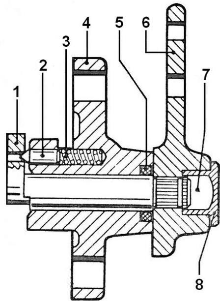
Press the shift control lever on to the shifter shaft so that the shift control lever is placed in neutral position at  $90^{\circ} \pm 30'$  to the gear shaft length.
